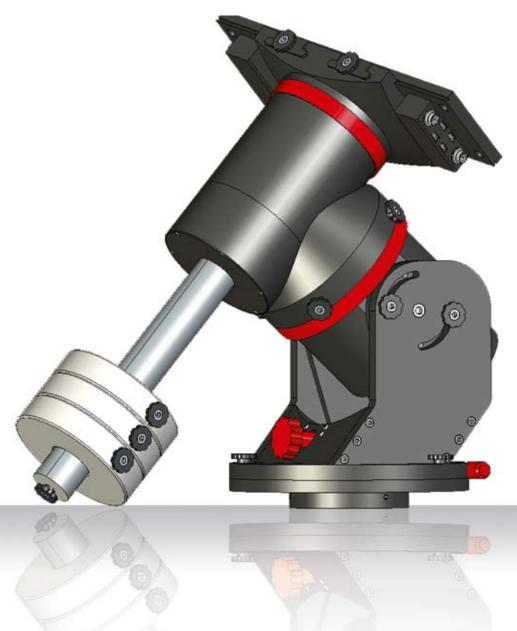
The ASA Direct Drive Mount 85 (ASA DDM85) is a robotic high-end mount, which can be operated without conventional guiding controls, due to its high accuracy. By the use of a gearless drive and high-resolution encoders it can achieve a tracking precision in the range of a tenth of an arc-second.
