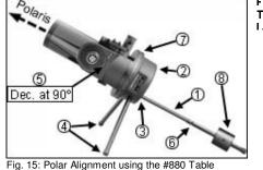
Fig. 15: Polar Alignment using the #880 Table Tripod. (1) Standard Tripod Leg with Latitude Scale; (2) High Latitude Hole; (3) Alternate Hole; (4) Fixed Tripod Legs; (5) Declination Pointer; (6) Thumbscrew; (7) R.A. Scale Pointer; (8) optional #1422 Low-Latitude Balance Weight. Fig. 14: Standard Tripod Leg: Latriude Scales
