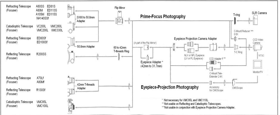
Note: If your purchase of the Vixen refracting telescope or catadioptric telescope does not come with the flip mirror, a complete set of 60mm thread-diameter extension tube, downsizing ring and 42mm to 31.7mm eyepiece adapter may be needed to attach the eyepiece projection camera adapter.
